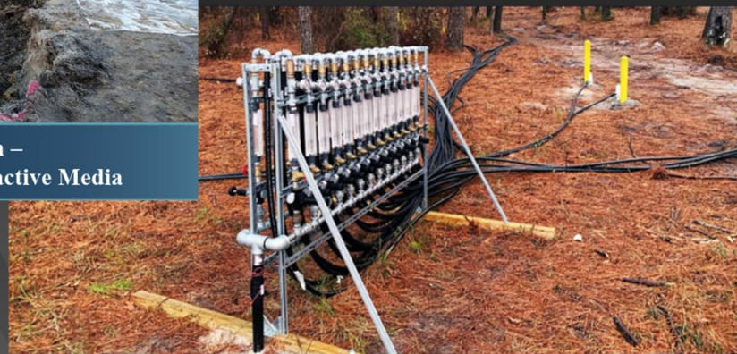
Air Sparging Manifold at Site 82
