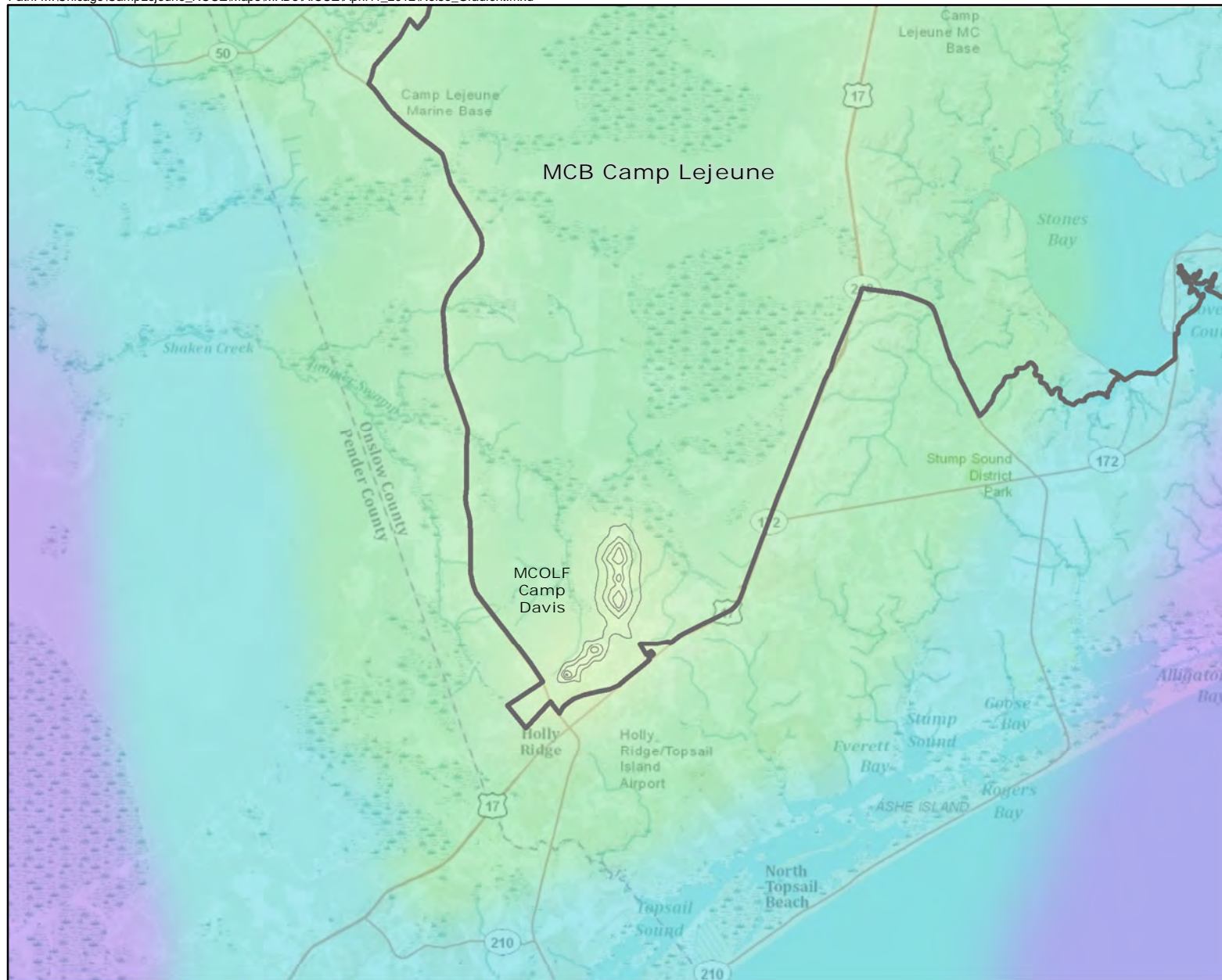
Figure 4-3 Estimate of Noise Propagation from Operations at MCOLF Camp Davis North Carolina
