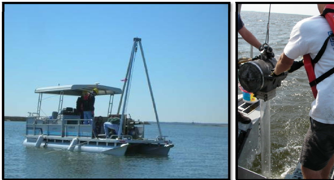
Figure 4. A pontoon boat retrofitted with a vibracore (left) was used to collect sediment samples in polycarbonate tubes (right).
