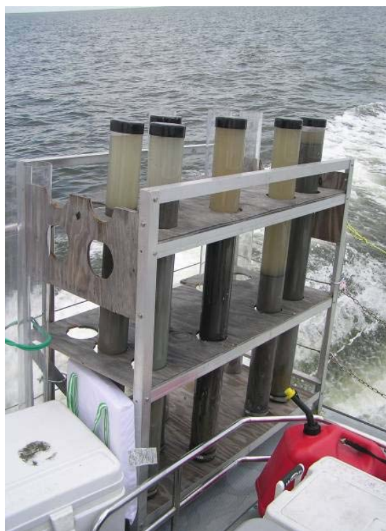
Figure 5. Vertical stowage of sediment in capped sampling tubes, awaiting post-processing.
