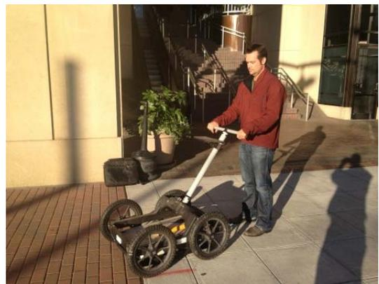
During the survey, the team may mark locations in the yard with paint or pin flags. The markings simply notify the team of a potential UST, so that its location may be documented. Please do not alter the markings. Subsequently, a probe will be used to identify the depth of the possible UST, and a minor disturbance to the landsurface may be observed in the survey area. The pin flags will be removed when the individual survey is complete.
